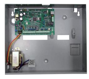
The ICP-CC408 Control Panel provides eight programmable zones.
